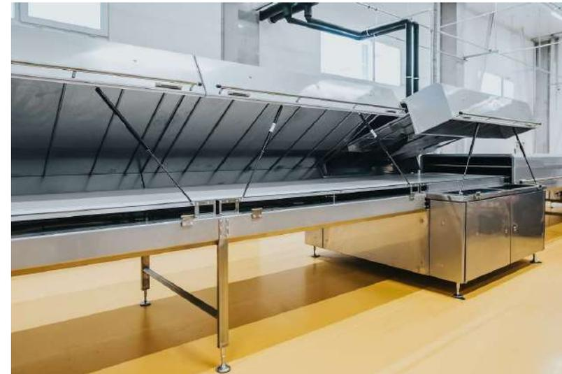
....open cooling conveyors / for ambient cooling / are also available
